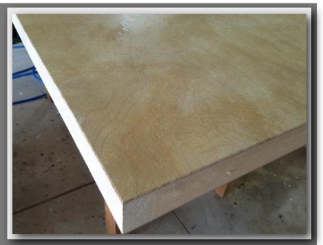
Spray, roller or brush contact adhesive evenly across the appropriate face of the door core. Insure that you cover 100% of each surface and leave to dry.
