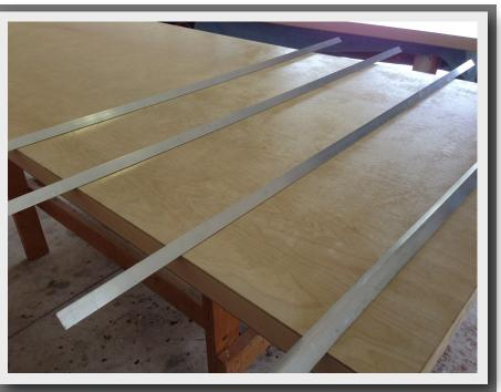
Place separator sticks on the substrate and then lay the veneer on the separator sticks taking care to insure the glued surfaces do not touch.
