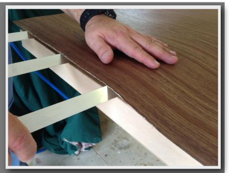
Remove the separator sticks one by one and smooth out the veneer working from the center outwards. Insure the veneer is pressed firmly down using a straight edge and any air expelled.
