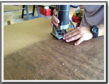
Using a high speed router, trim the excess veneer from the edges of the substrate.
