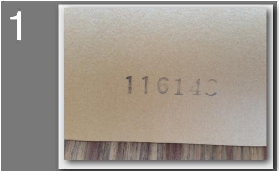
Locate the flitch # (in this case 116148) on the bottom of back of the sheet . Insure that the sheet you are about to bond is from the correct flitch.
