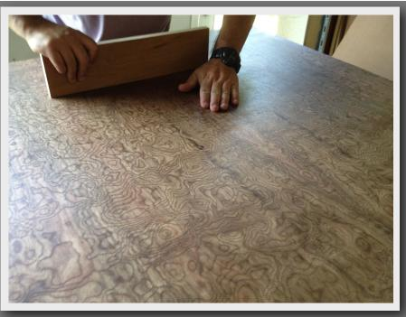
Remove the separator sticks one by one and smooth out the veneer working from the center outwards. Insure the veneer is pressed firmly down and any air expelled.
