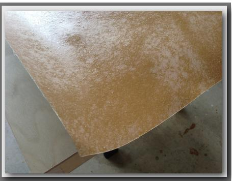
Spray, roller or brush contact adhesive evenly across the back surface of the veneer. Insure that you cover 100% of each surface and leave to dry.
