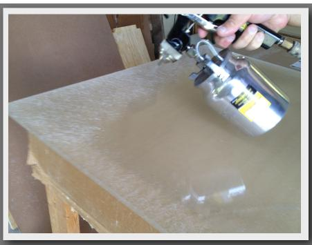
Spray, roller or brush 3M-4693H adhesive evenly across the two surfaces to be bonded together. Insure that you cover 100% of each surface and leave to dry.
